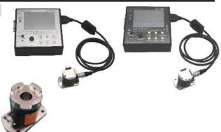
**Detector which is down sized for automation facility** Enable to choose the indicator to suit the usage scene
